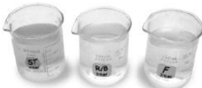
Septic Tank Recirc/Blend Filtrate
